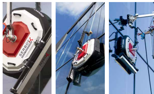
GEKKO Facade Cleaning Robot GEKKO Facade with Mono Rail GEKKO Facade with Boom Lift (from left to right)
